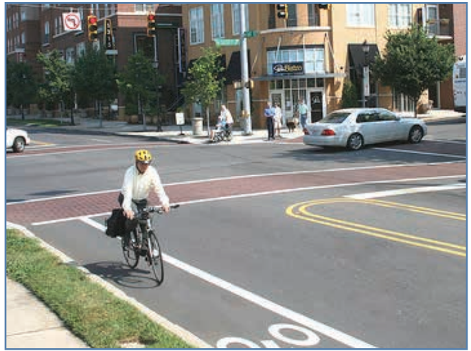
Example of an intersection that displays highly visible crosswalks, grassy planting strips, street trees, bike lanes, ADA-compliant curb cuts, and good pavement markings.
